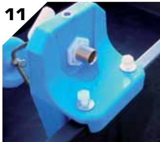
11 Place 2 nylon screws and s.steel washers through the holes in the ballcock support into the threaded holes in the trough wall.
