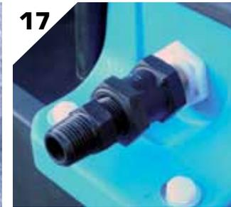
17 Place the assembly on the end of the float valve inlet. Align the threads correctly then tighten.
