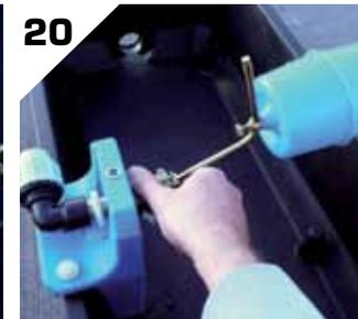
20 Engage the thread of the float valve inlet & elbow fitting and rotate the float valve assembly to tighten.
