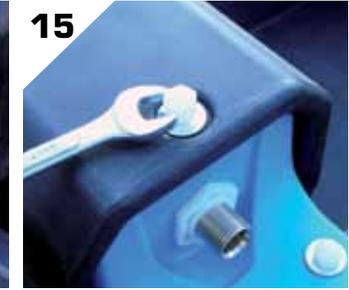
15 Place a nylon screw and a s.steel washer through the hole on top of the ballcock cover into the threaded hole on the ballcock support below. Then tighten.
